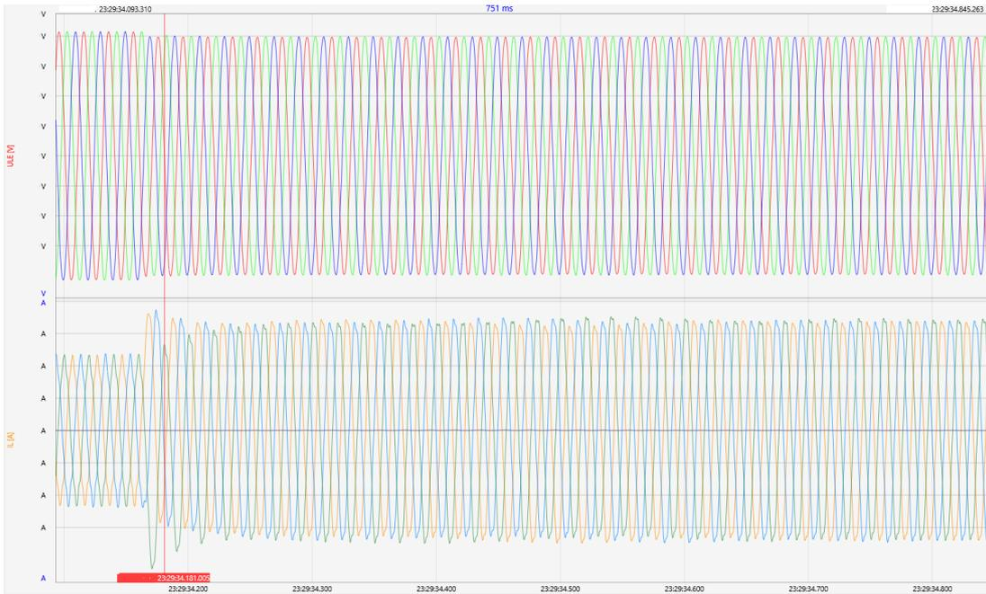
**Figure 3.5:** Example of voltage and current measurement when switching on load
