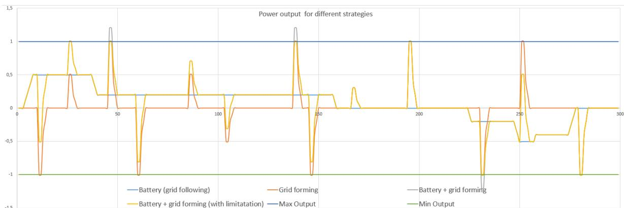
**Figure 3.33:** Power output of an inverter providing different services.
