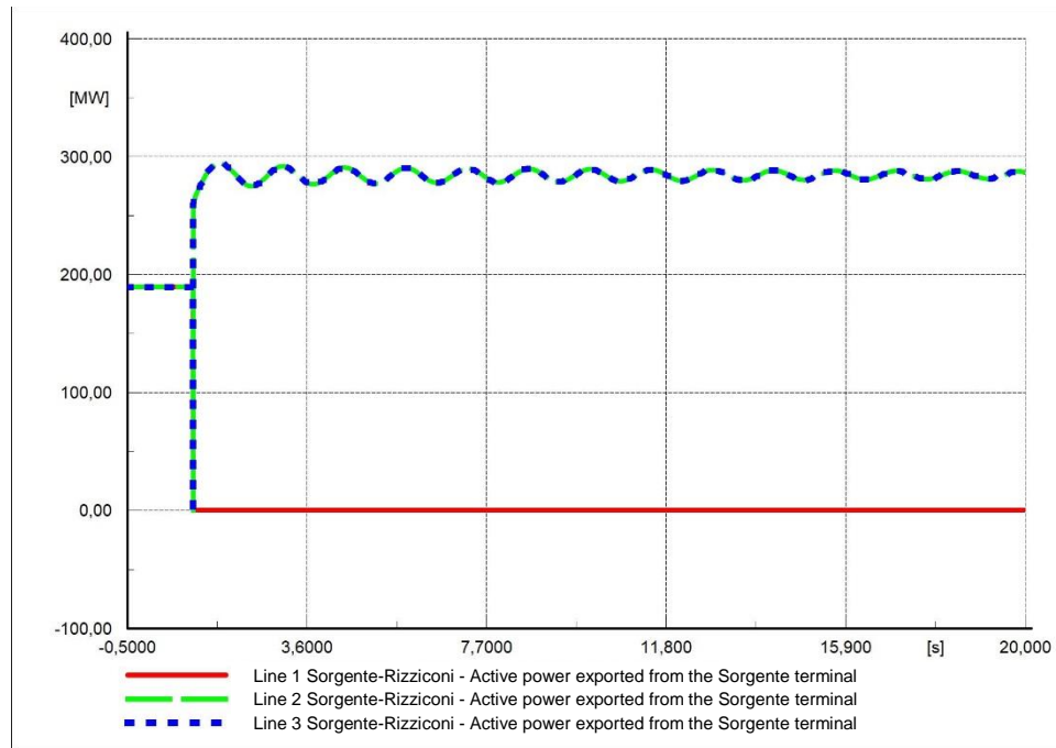
Figure 6. Network: 2030. Dispatching profile: High Export, Event: outage of one of the three connections with continental Italy, No-SI-Wind configuration. Power exported from the Sorgente terminal through the three connections with continental Italy.
