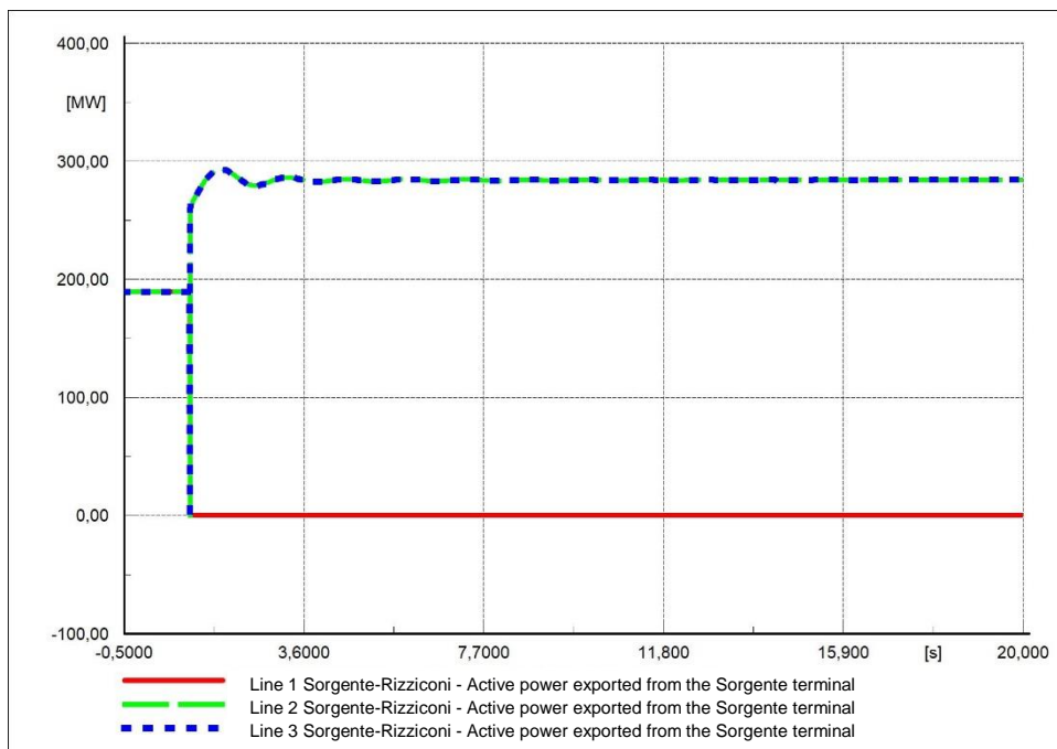
Figure 5. Network: 2030. Dispatching profile: High Export, Event: outage of one of the three connections with continental Italy, base configuration. Power exported from the Sorgente terminal through the three connections with continental Italy.
