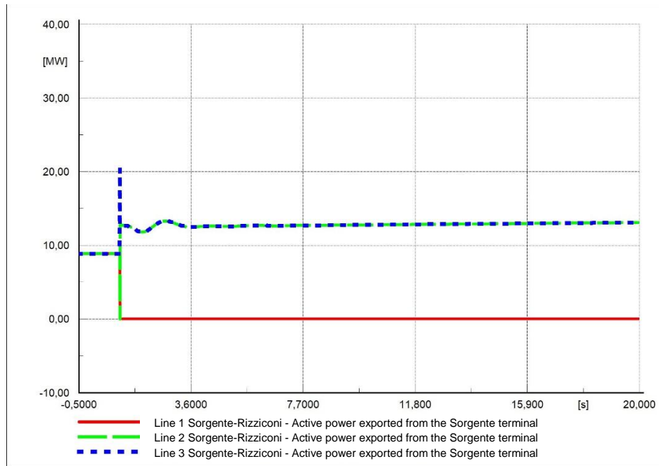
Figure 33. Network: 2030. Dispatching profile: High Load / Low Gas, Event: outage of one of the three connections with continental Italy, No-SI-Wind configuration. Power exported from the Sorgente terminal through the three connections with continental Italy.
