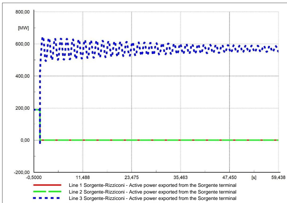
Figure 10. Network: 2030. Dispatching profile: High Export, Event: outage of two of the three connections with continental Italy, No-SI-Wind configuration. Power exported from the Sorgente terminal through the three connections with continental Italy.
