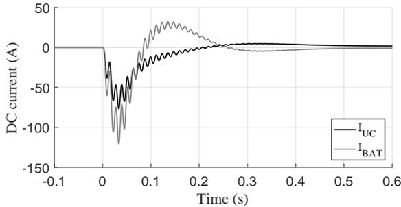
Fig. 5. DC current following load disconnection with VRC
