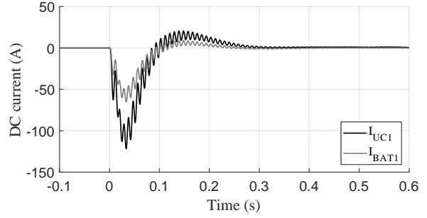
Fig. 6. DC current following load disconnection with PIP
