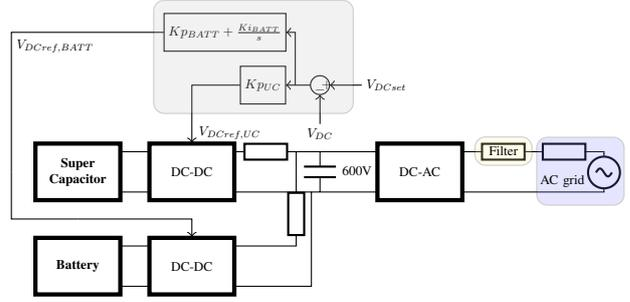
Fig. 2. PIP controller for DC side power sharing
