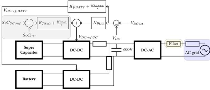
Fig. 4. PI controller for ultracap SoC regulation
