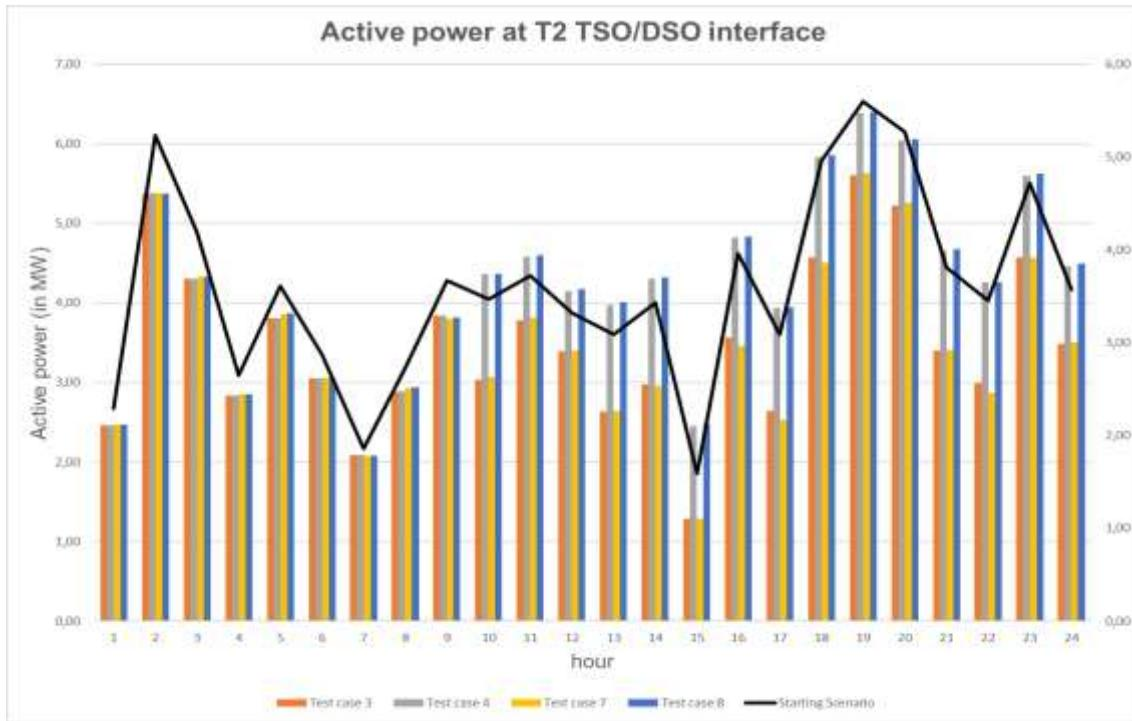
Figure 5-21 – Active Power profile at T2 TSO/DSO interface for cluster 2 test cases
