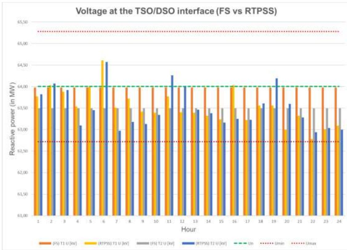
Figure 5-55 – Voltage results at TSO/DSO interface for test case 14
