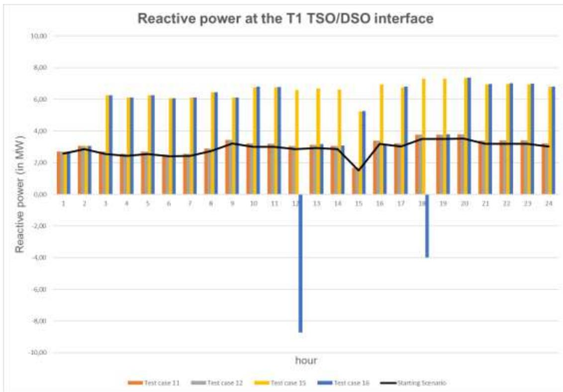
Figure 5-58 – Reactive Power profile at T1 TSO/DSO interface for cluster 4 test cases
