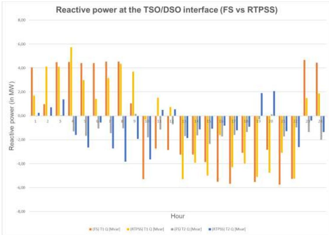
Figure 5-36 – Reactive Power results at TSO/DSO interface for test case 8
