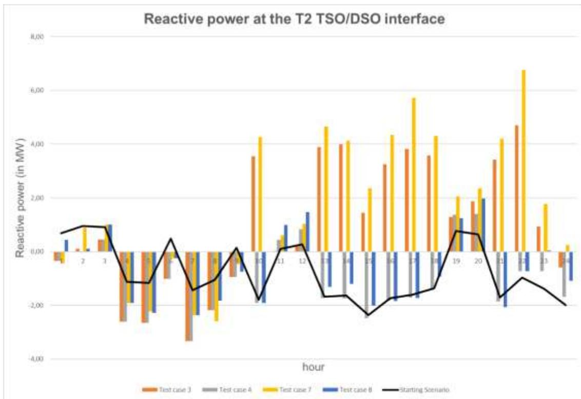
Figure 5-23 – Reactive Power profile at T2 TSO/DSO interface for cluster 2 test cases
