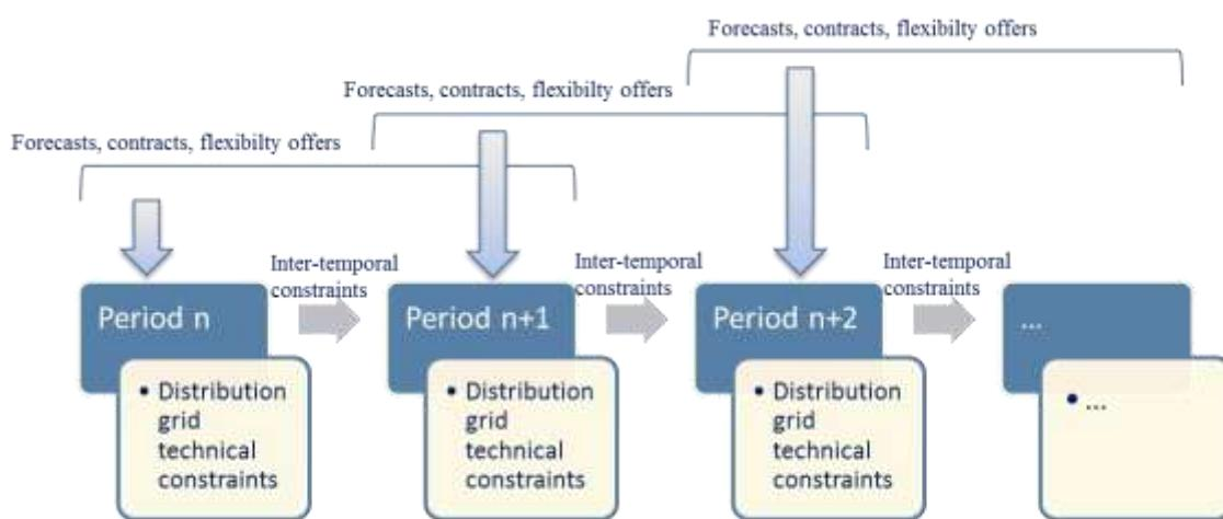
**Figure 3-4 – Sequence-constrained OPF (ScOPF) using a moving window approach.**
