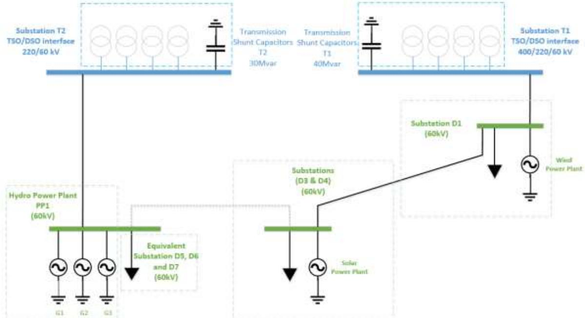
Figure 4-10 – RTPSS distribution network representation (meshed operation)
