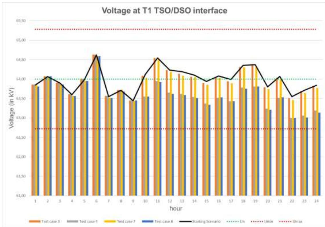
Figure 5-24 – Voltage at T1 TSO/DSO interface for cluster 2 test cases
