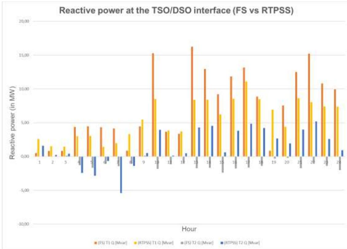
Figure 5-15 – Reactive Power results at TSO/DSO interface for test case 5
