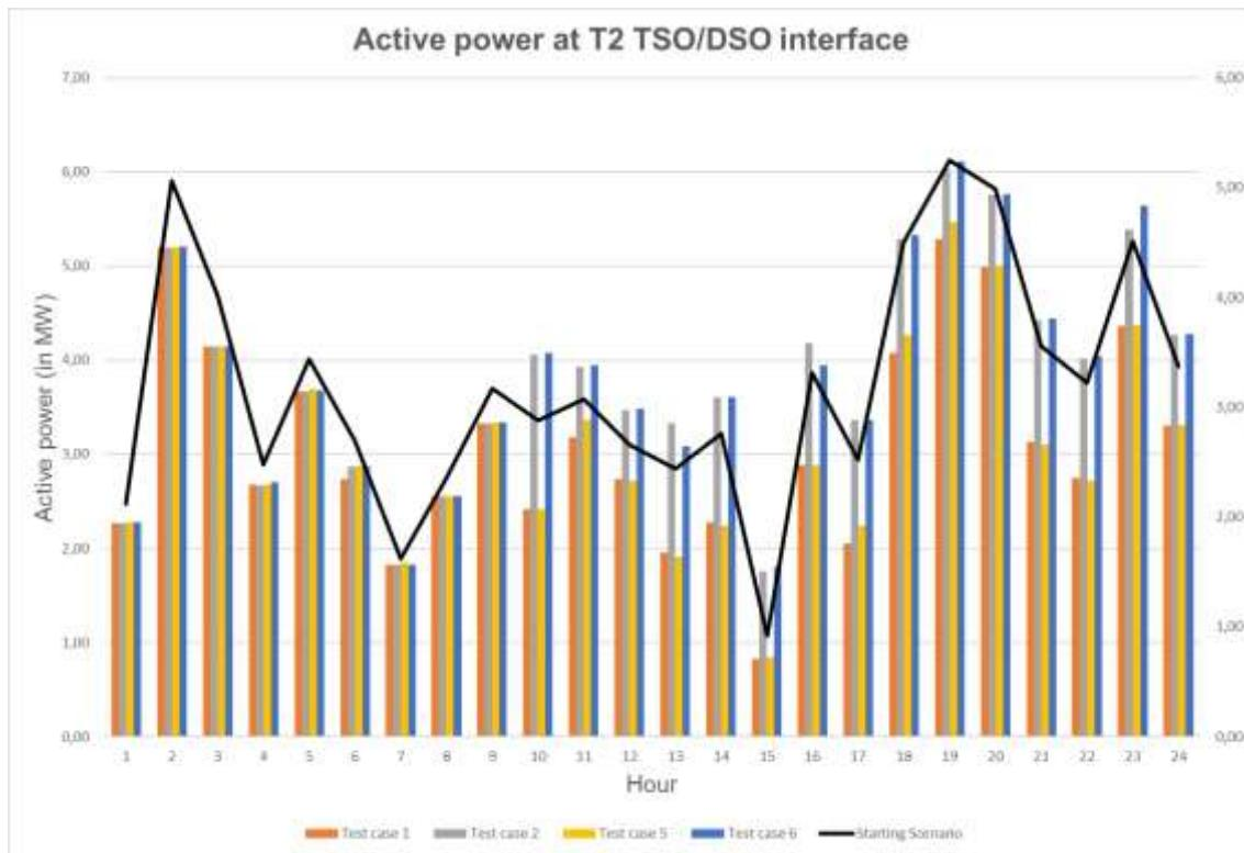
Figure 5-3 – Active Power profile at T2 TSO/DSO interface for cluster 1 test cases
