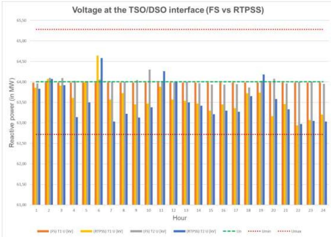
Figure 5-13 – Voltage results at TSO/DSO interface for test case 2
