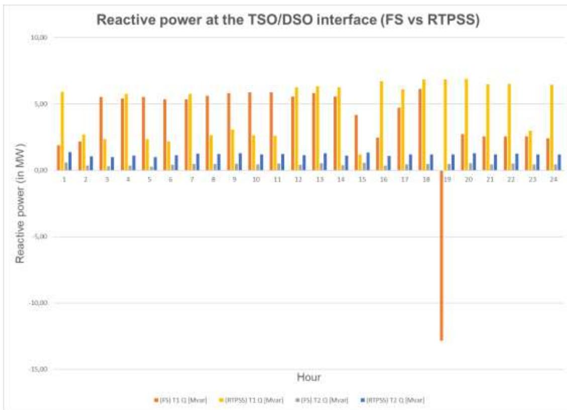
Figure 5-54 – Reactive Power results at TSO/DSO interface for test case 14
