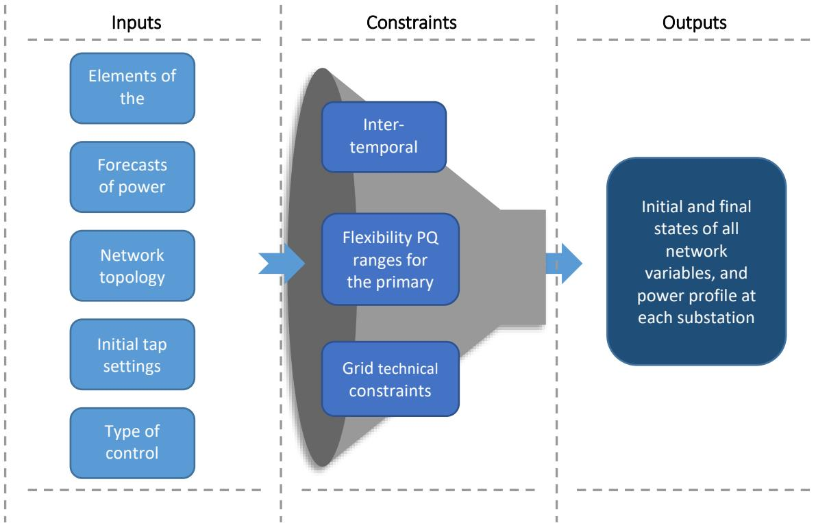
Figure 3-5 – Inputs and outputs of the ScOPF tool.
