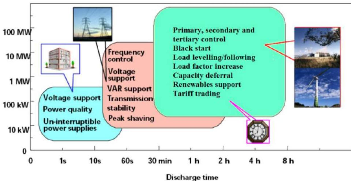
Figure 2-2 – Power ratings and discharge times required for different types of network services.
