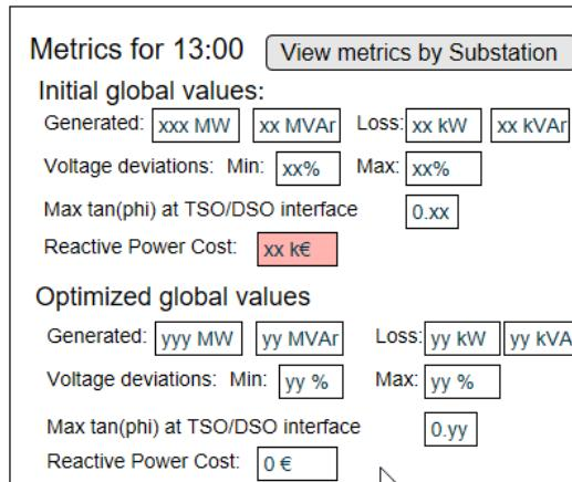
Figure 2-17 – Proposed GUI for “Metrics before and after optimization at an instant”
