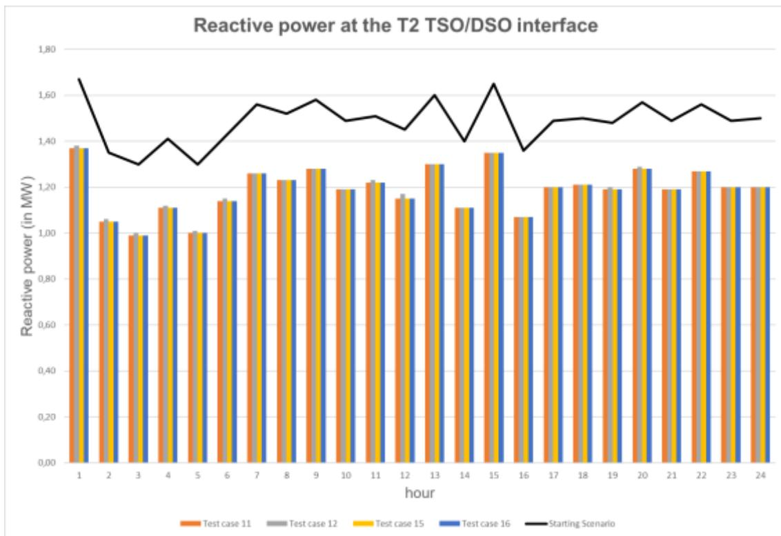
Figure 5-59 – Reactive Power profile at T2 TSO/DSO interface for cluster 4 test cases
