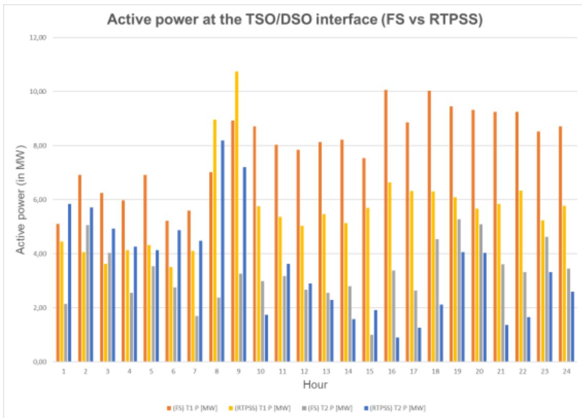
**Figure 5-14 – Active Power results at TSO/DSO interface for test case 5**
