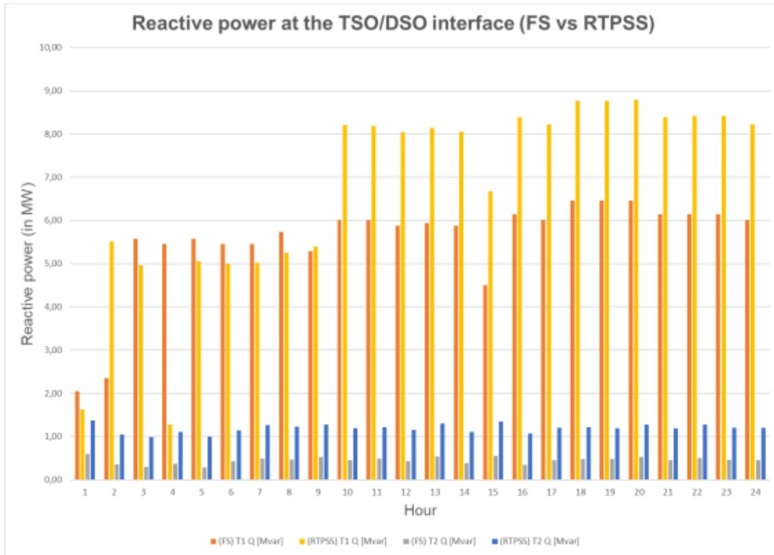
Figure 5-69 – Reactive Power results at TSO/DSO interface for test case 15
