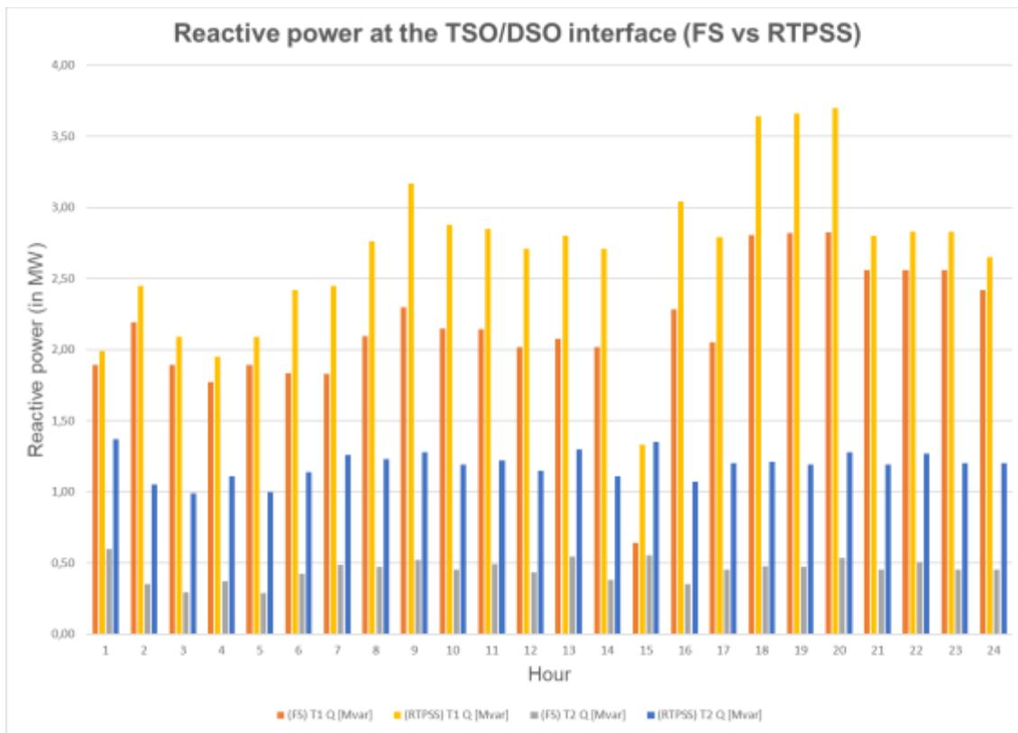
Figure 5-48 – Reactive Power results at TSO/DSO interface for test case 10
