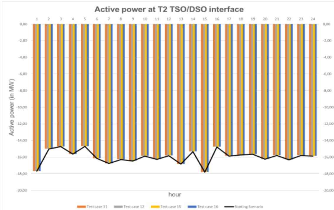
Figure 5-57 – Active Power profile at T2 TSO/DSO interface for cluster 4 test cases
