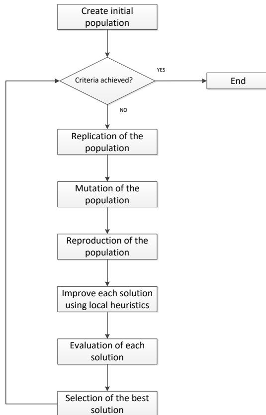
**Figure 3-3 – Heuristic methodology to solve the ScOPF.**
