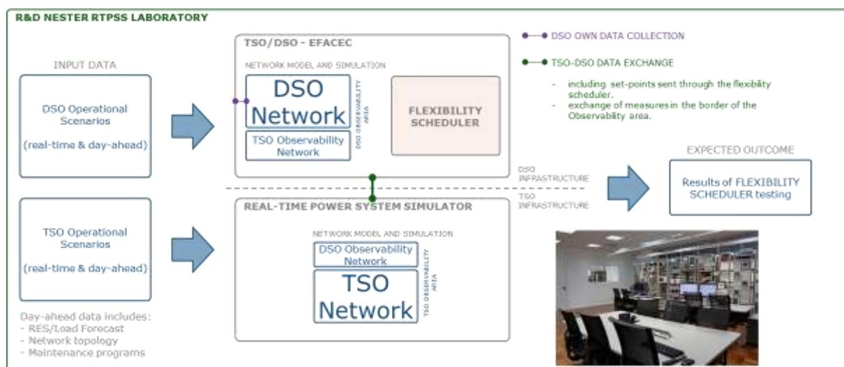
**Figure 2-19 – Architecture to be implemented in the R&D Nester RTPSS Laboratory for the sub-task 7.2.3**
