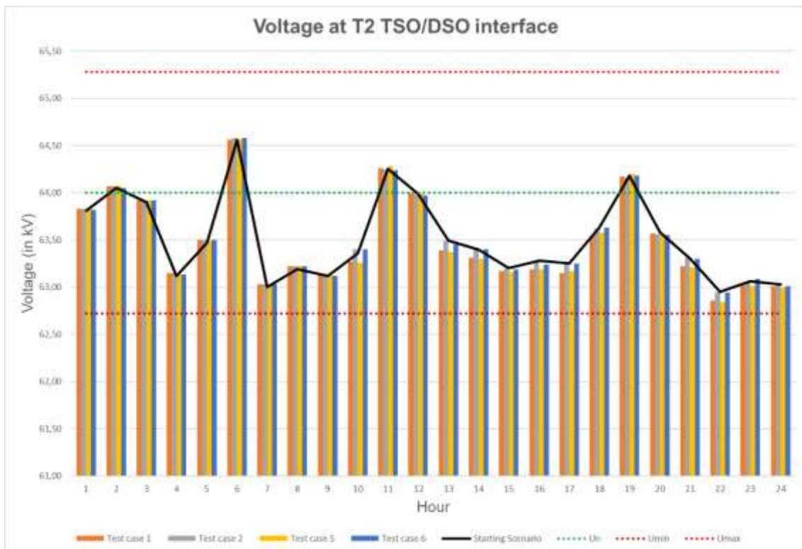
Figure 5-7 – Voltage at T2 TSO/DSO interface for cluster 1 test cases
