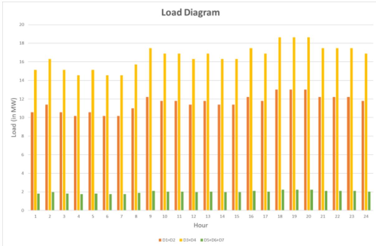
**Figure 4-4 – Load diagram of the distribution substations' subsets**
