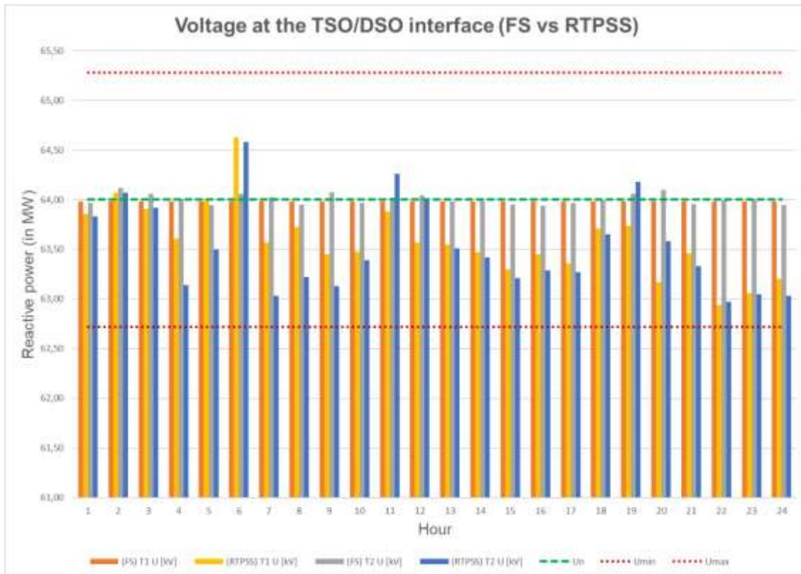
Figure 5-31 – Voltage results at TSO/DSO interface for test case 4
