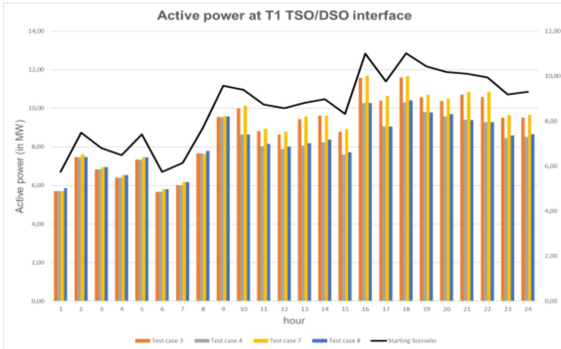
Figure 5-20 – Active Power profile at T1 TSO/DSO interface for cluster 2 test cases
