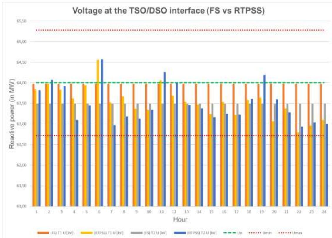
Figure 5-73 – Voltage results at TSO/DSO interface for test case 16
