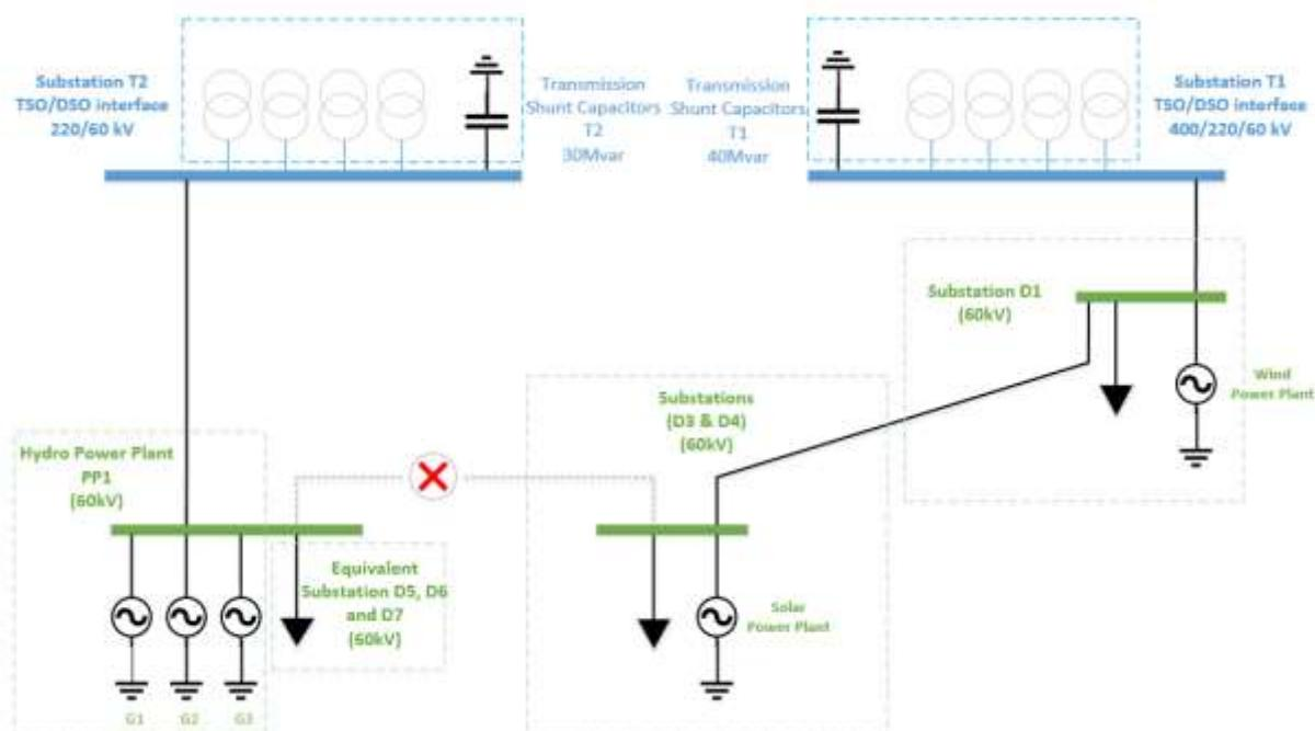
Figure 4-11 – RTPSS distribution network representation (radial operation)
