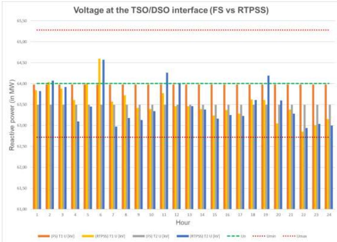
Figure 5-49 – Voltage results at TSO/DSO interface for test case 10
