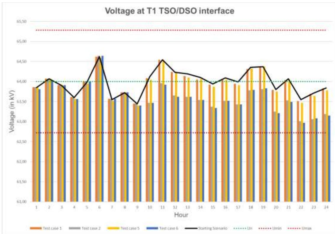
Figure 5-6 – Voltage at T1 TSO/DSO interface for cluster 1 test cases
