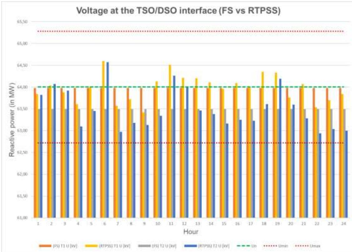
Figure 5-46 – Voltage results at TSO/DSO interface for test case 9
