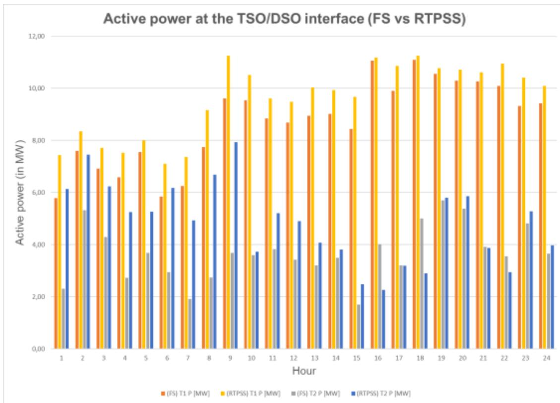
Figure 5-32 – Active Power results at TSO/DSO interface for test case 7
