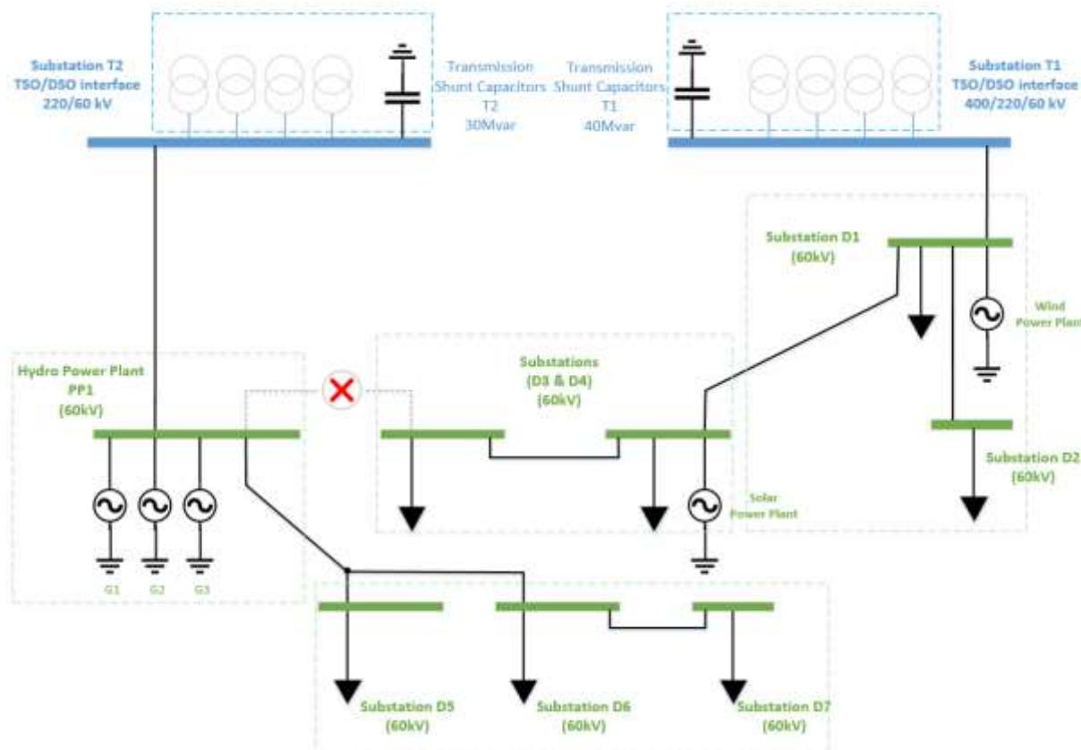
Figure 4-8 – Flexibility Scheduler network representation (with open mesh)
