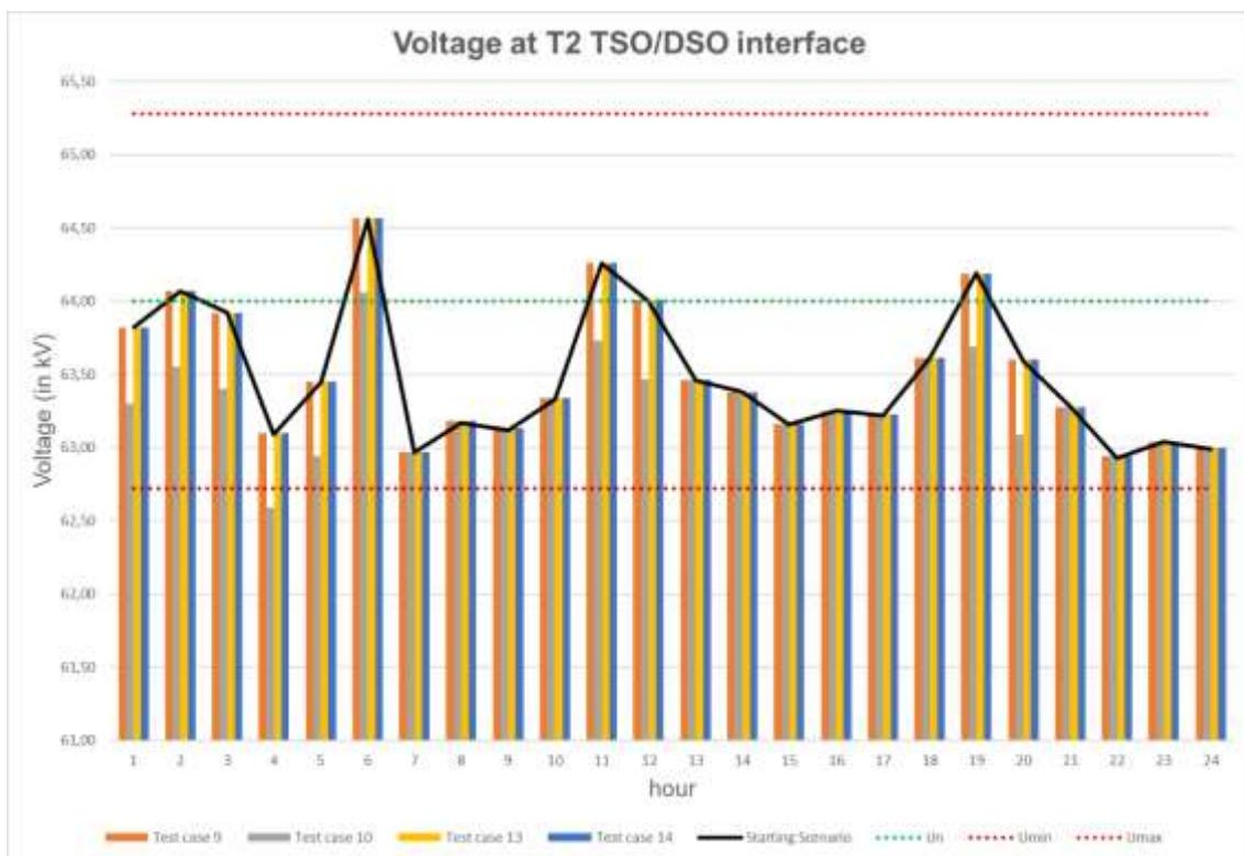
Figure 5-43 – Voltage at T2 TSO/DSO interface for cluster 3 test cases
