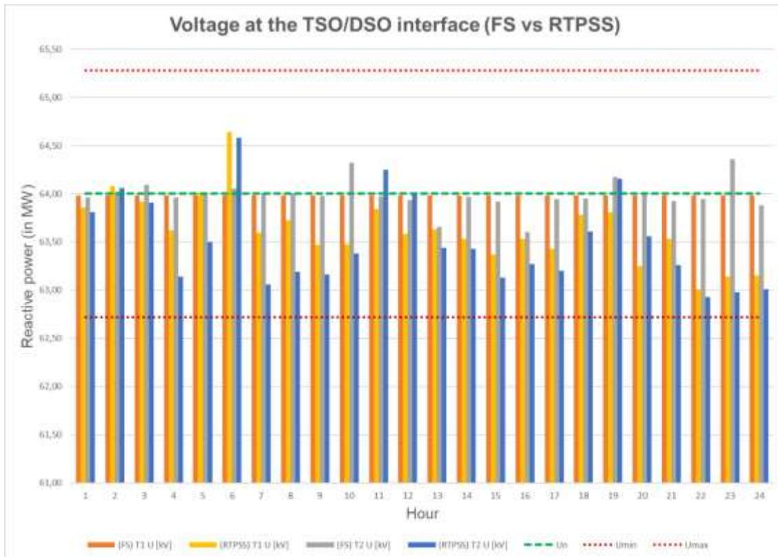
Figure 5-19 – Voltage results at TSO/DSO interface for test case 6
