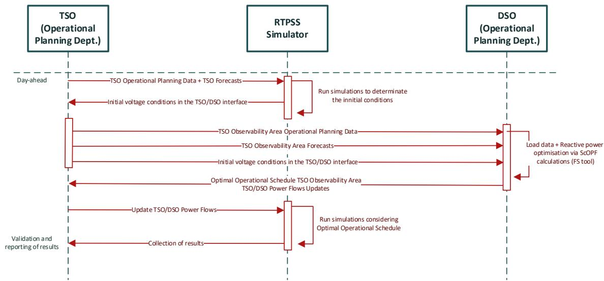
Figure 4-12 – Sequence diagram of the use case for the validation of the FS tool
