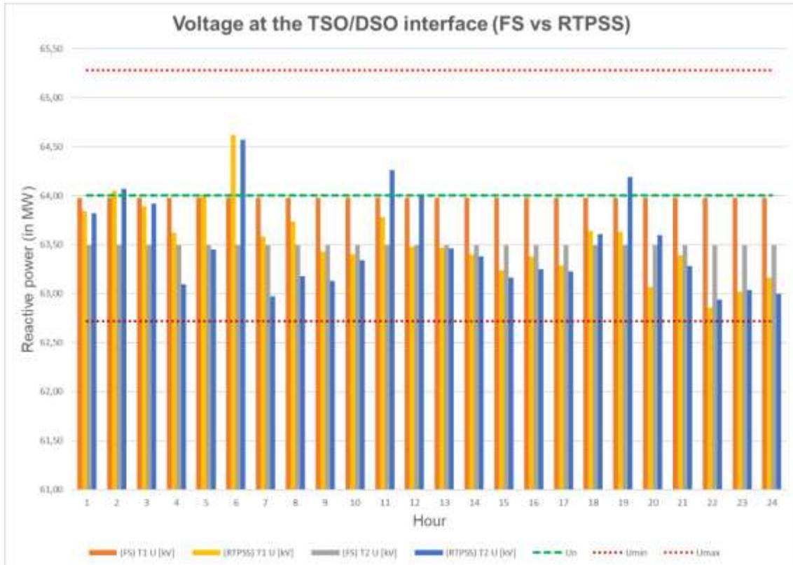
Figure 5-67 – Voltage results at TSO/DSO interface for test case 12
