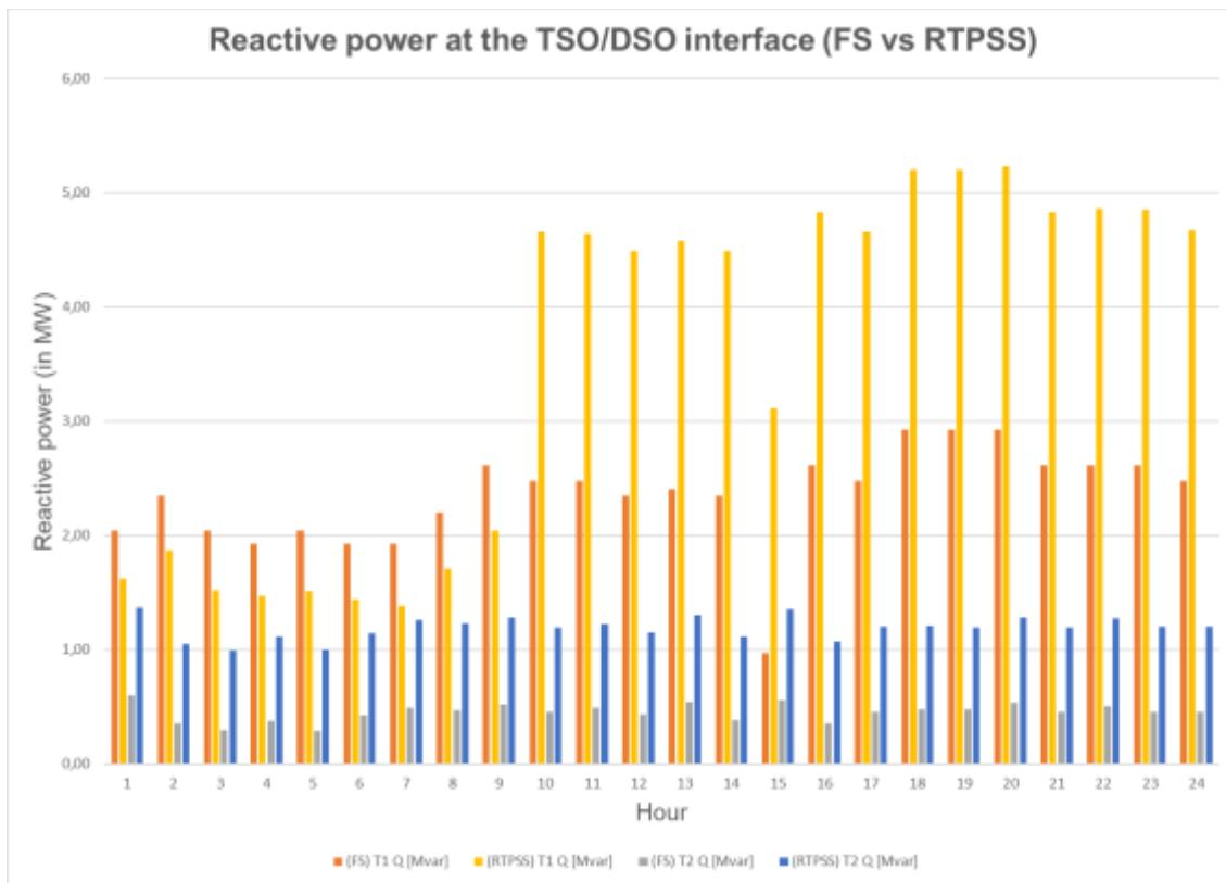
Figure 5-63 – Reactive Power results at TSO/DSO interface for test case 11
