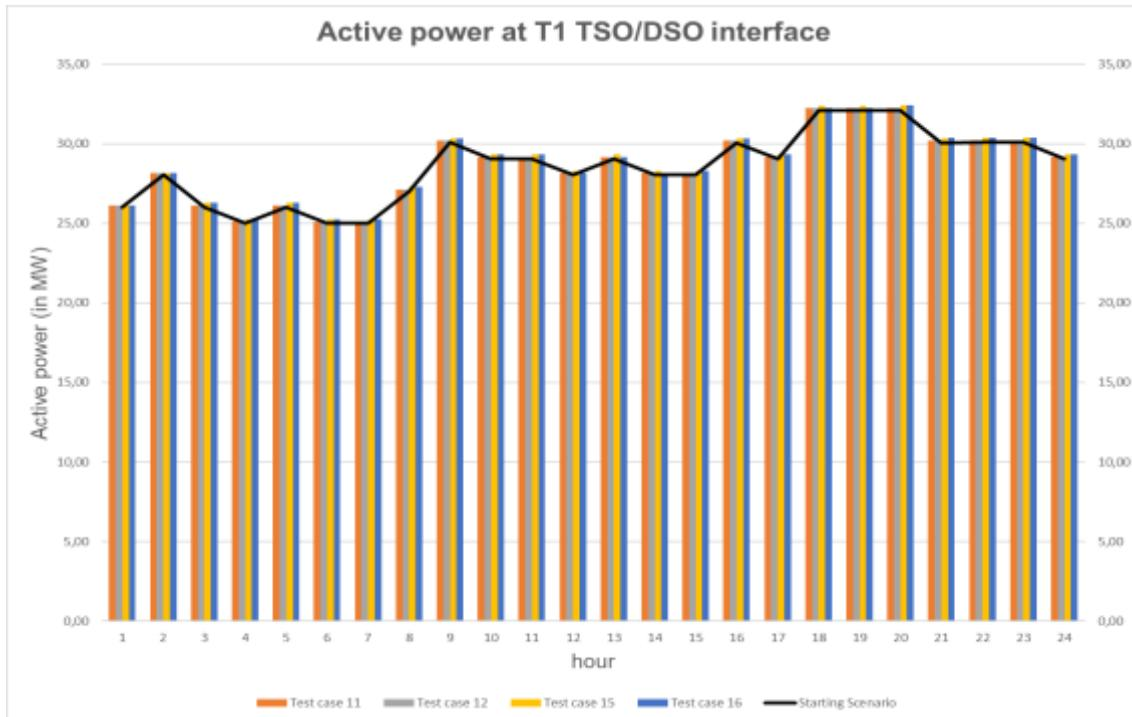
Figure 5-56 – Active Power profile at T1 TSO/DSO interface for cluster 4 test cases
