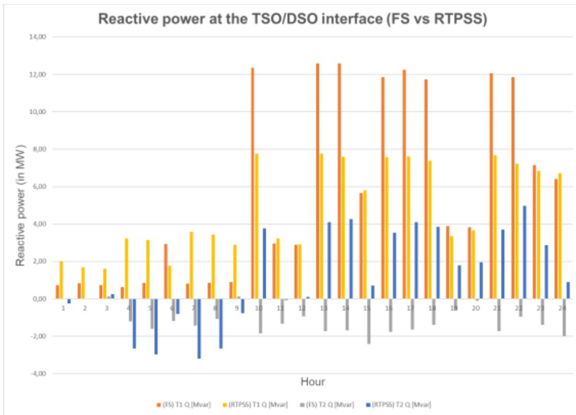
Figure 5-9 – Reactive Power results at TSO/DSO interface for test case 1
