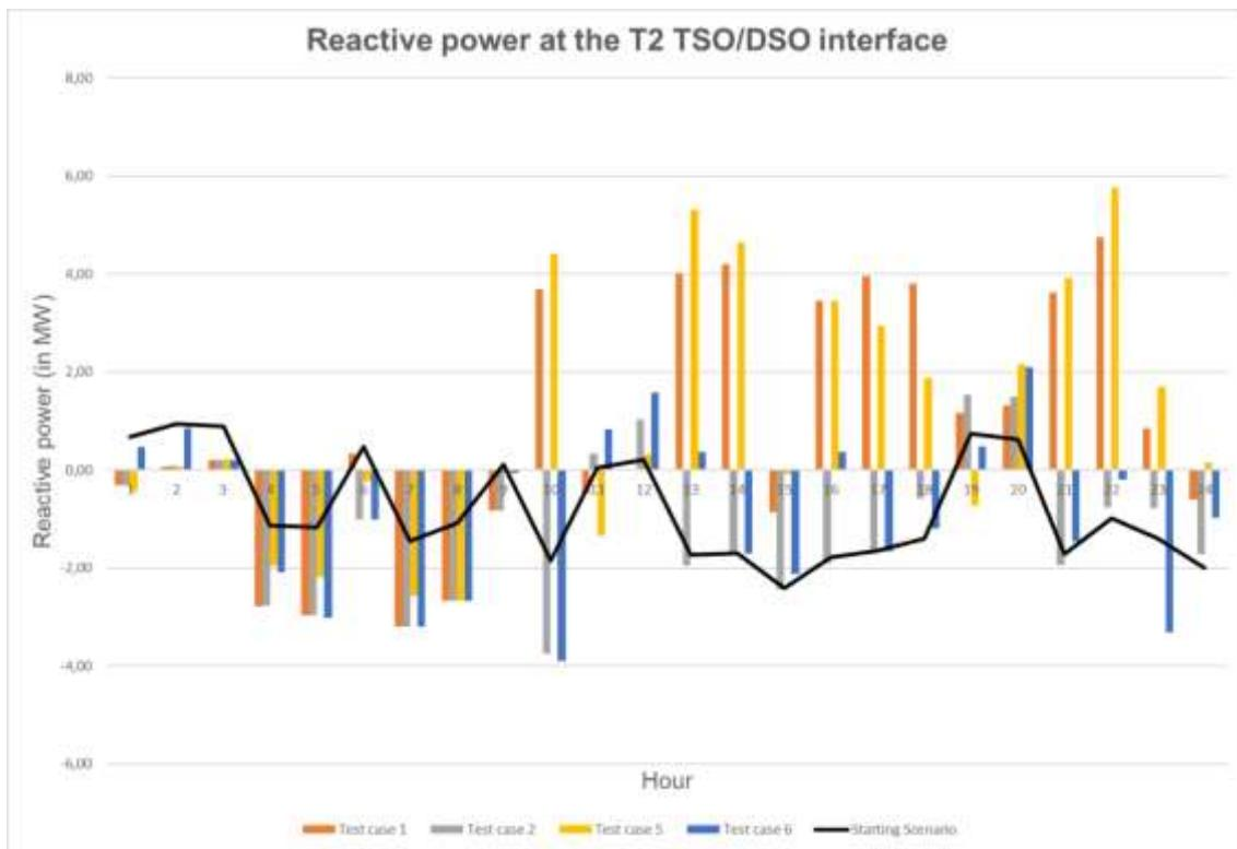
Figure 5-5 – Reactive Power profile at T2 TSO/DSO interface for cluster 1 test cases
