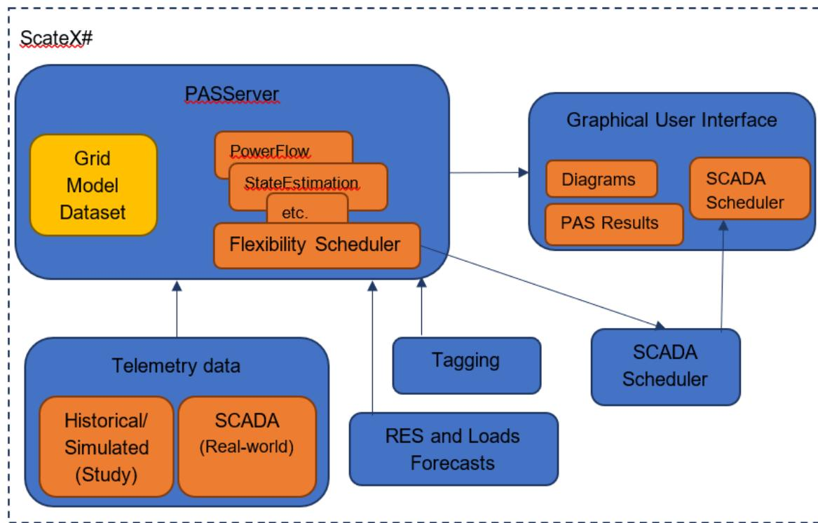
Figure 3-6 – Power applications architecture.
