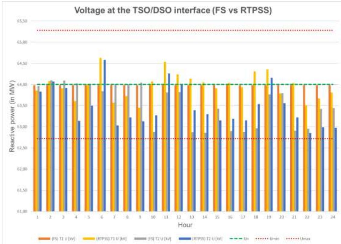
Figure 5-10 – Voltage results at TSO/DSO interface for test case 1
