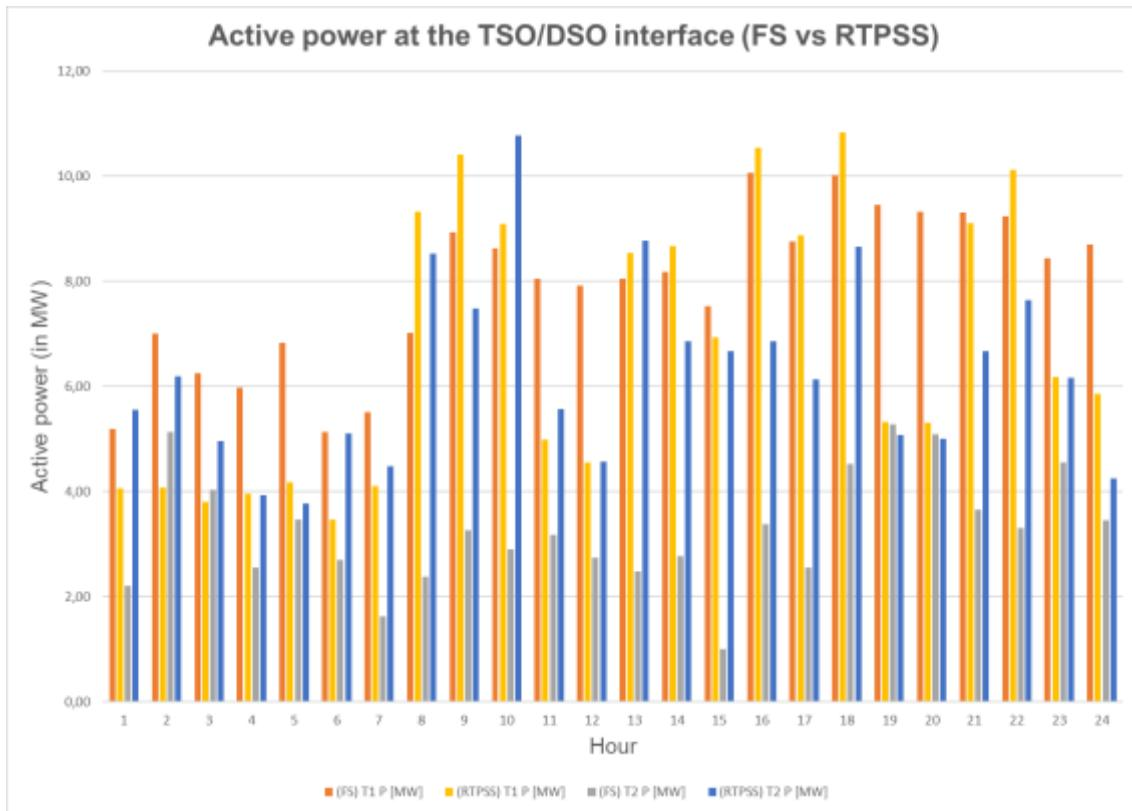
Figure 5-17 – Active Power results at TSO/DSO interface for test case 6
