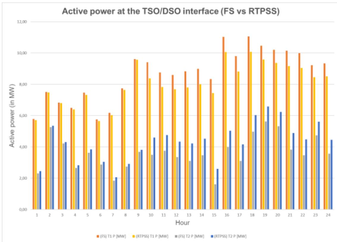
Figure 5-29 – Active Power results at TSO/DSO interface for test case 4
