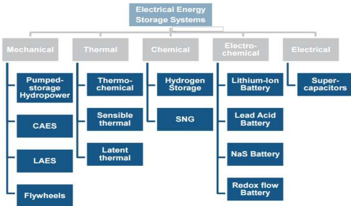
Figure 2-1 – Storage: different categories (FLEXNET)
