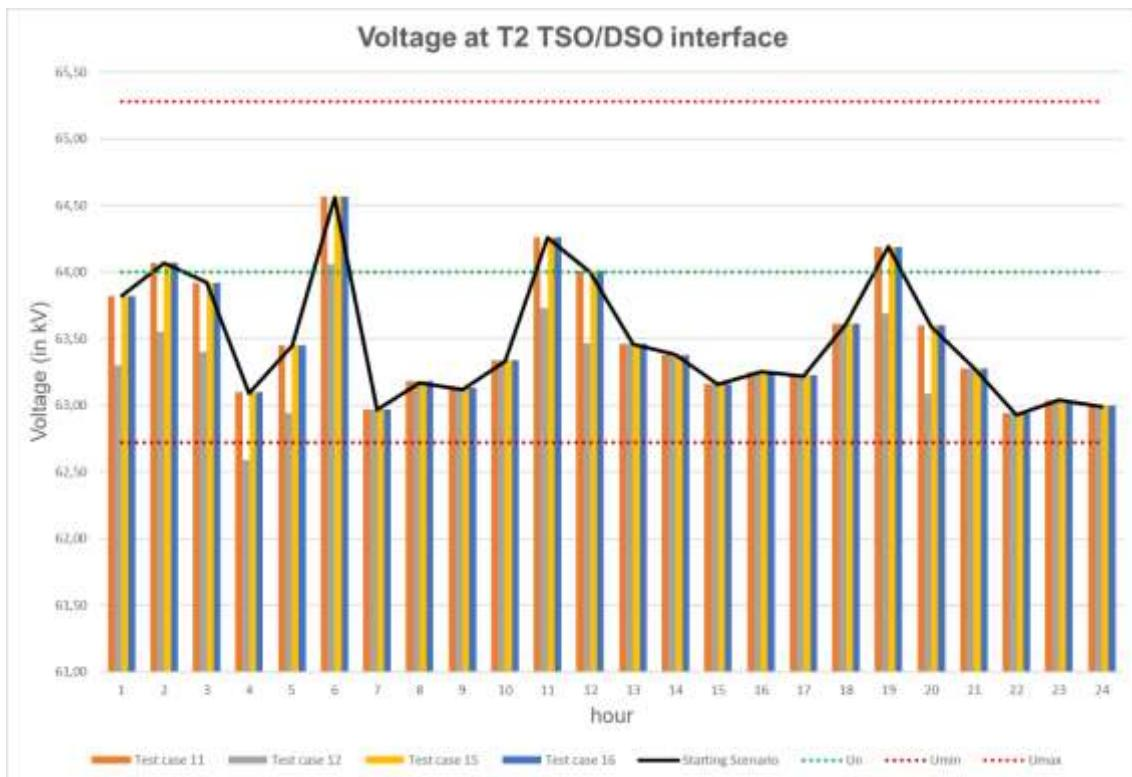
Figure 5-61 – Voltage at T2 TSO/DSO interface for cluster 4 test cases
