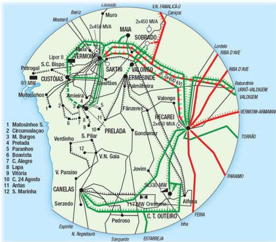
Figure 4-9 – Map of section of transmission grid modelled in RTPSS (Source: REE)
