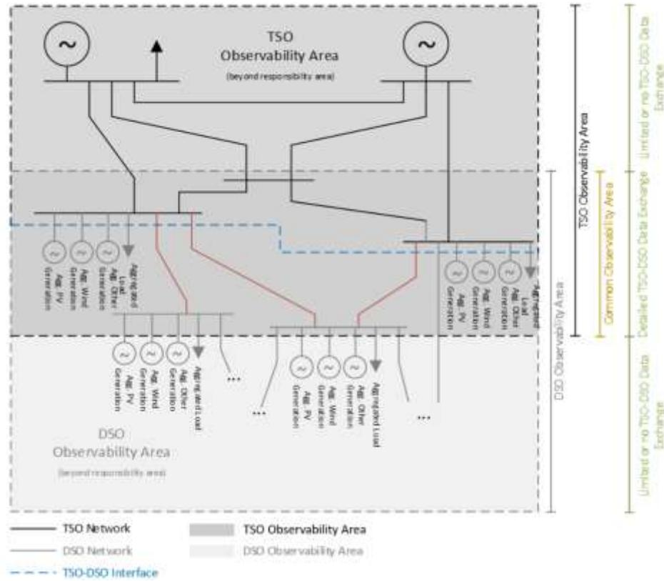
Figure 2-13 – The concept of observability area. Adapted from [22]
