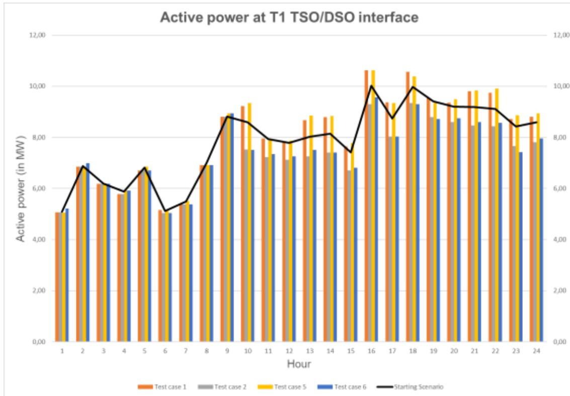
Figure 5-2 – Active Power profile at T1 TSO/DSO interface for cluster 1 test cases
