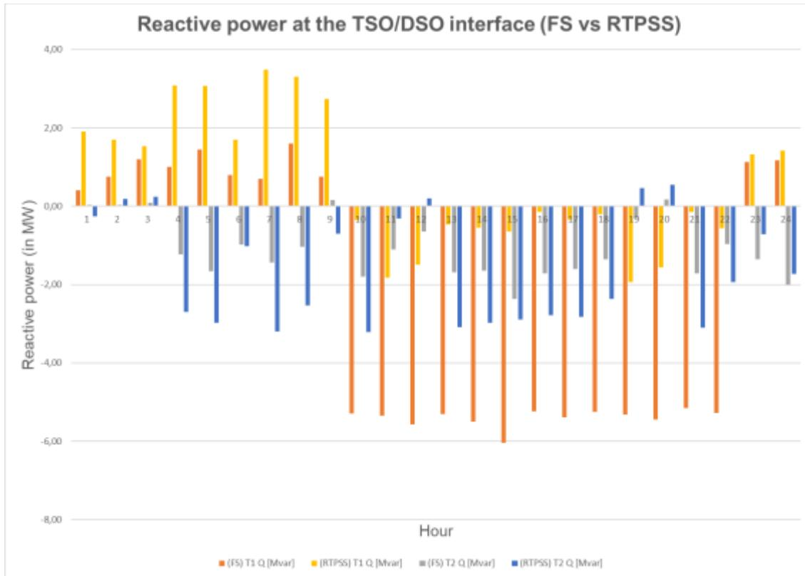
Figure 5-30 – Reactive Power results at TSO/DSO interface for test case 4
