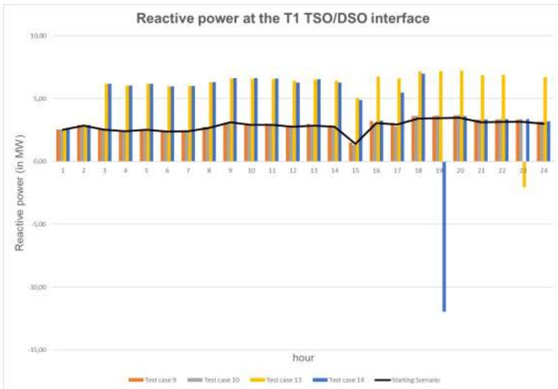
**Figure 5-40 – Reactive Power profile at T1 TSO/DSO interface for cluster 3 test cases**
