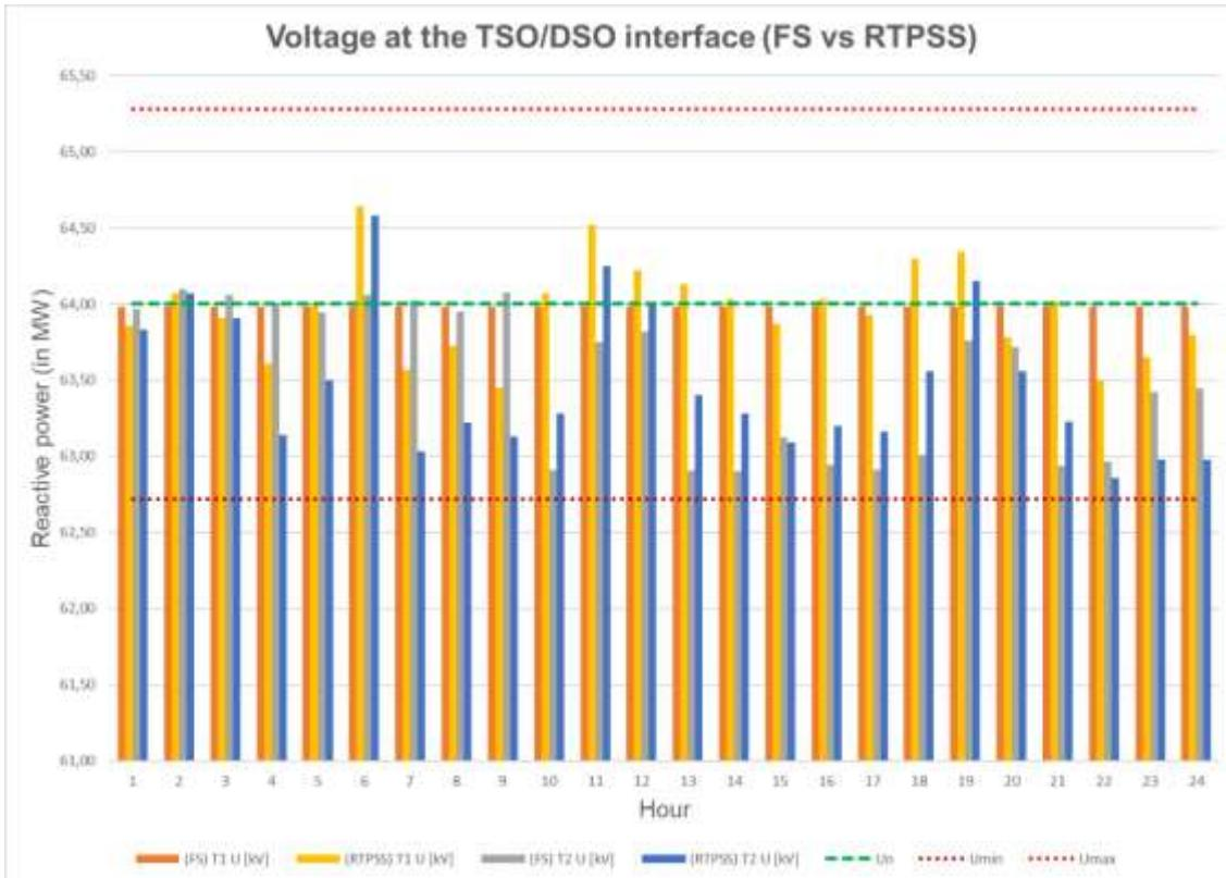
Figure 5-28 – Voltage results at TSO/DSO interface for test case 3
