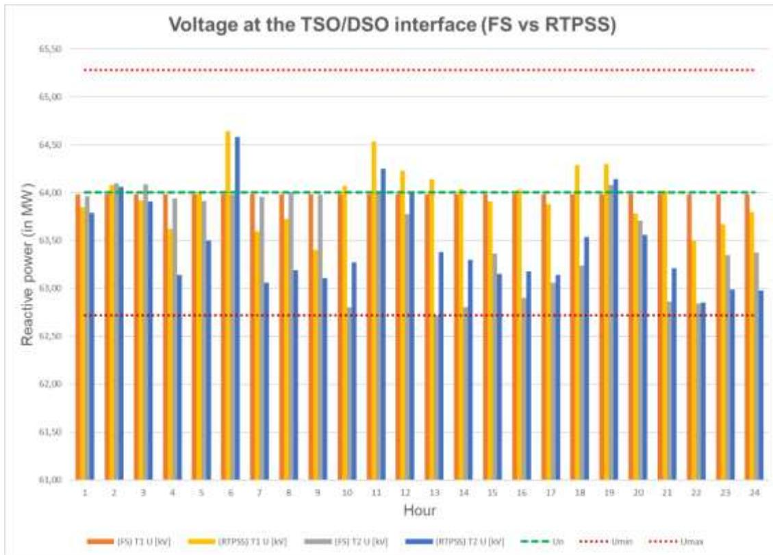
Figure 5-16 – Voltage results at TSO/DSO interface for test case 5
