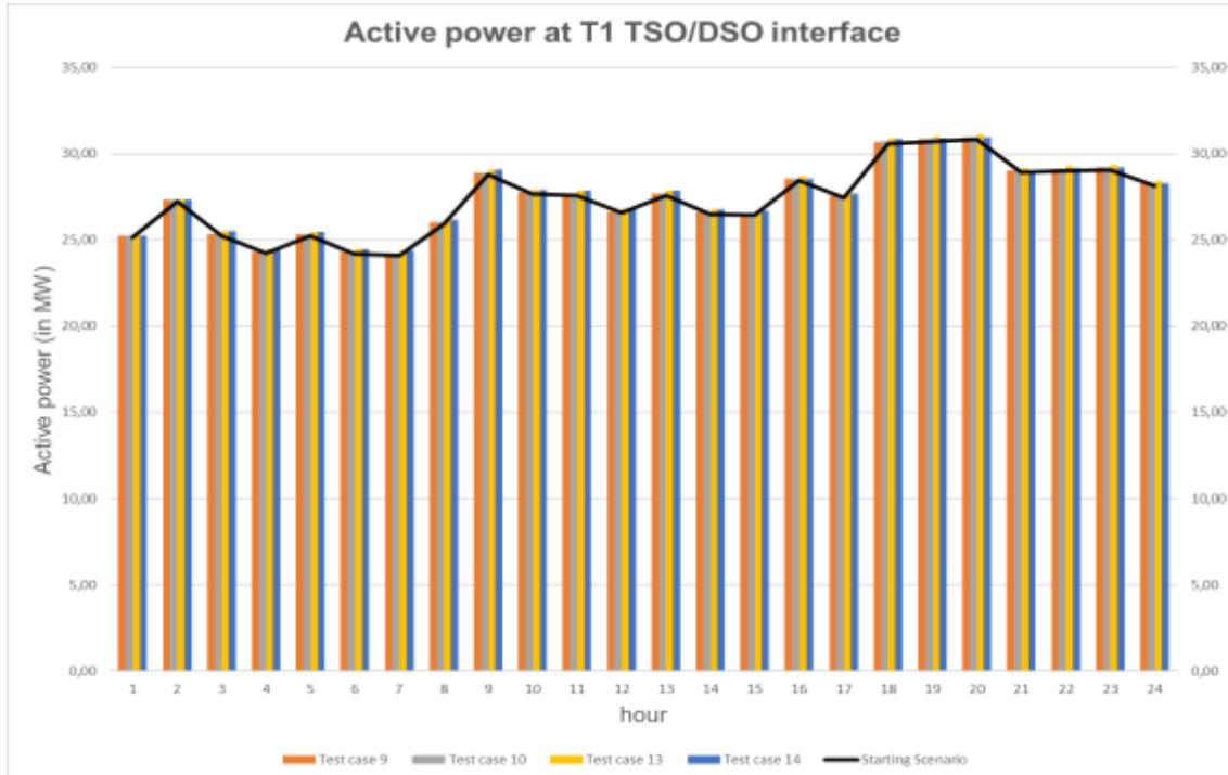
Figure 5-38 – Active Power profile at T1 TSO/DSO interface for cluster 3 test cases
