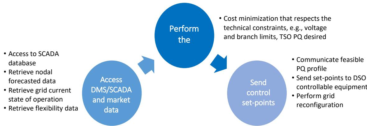
Figure 3-2 – High-level integration of the ScOPF in a monitoring and control infrastructure.
