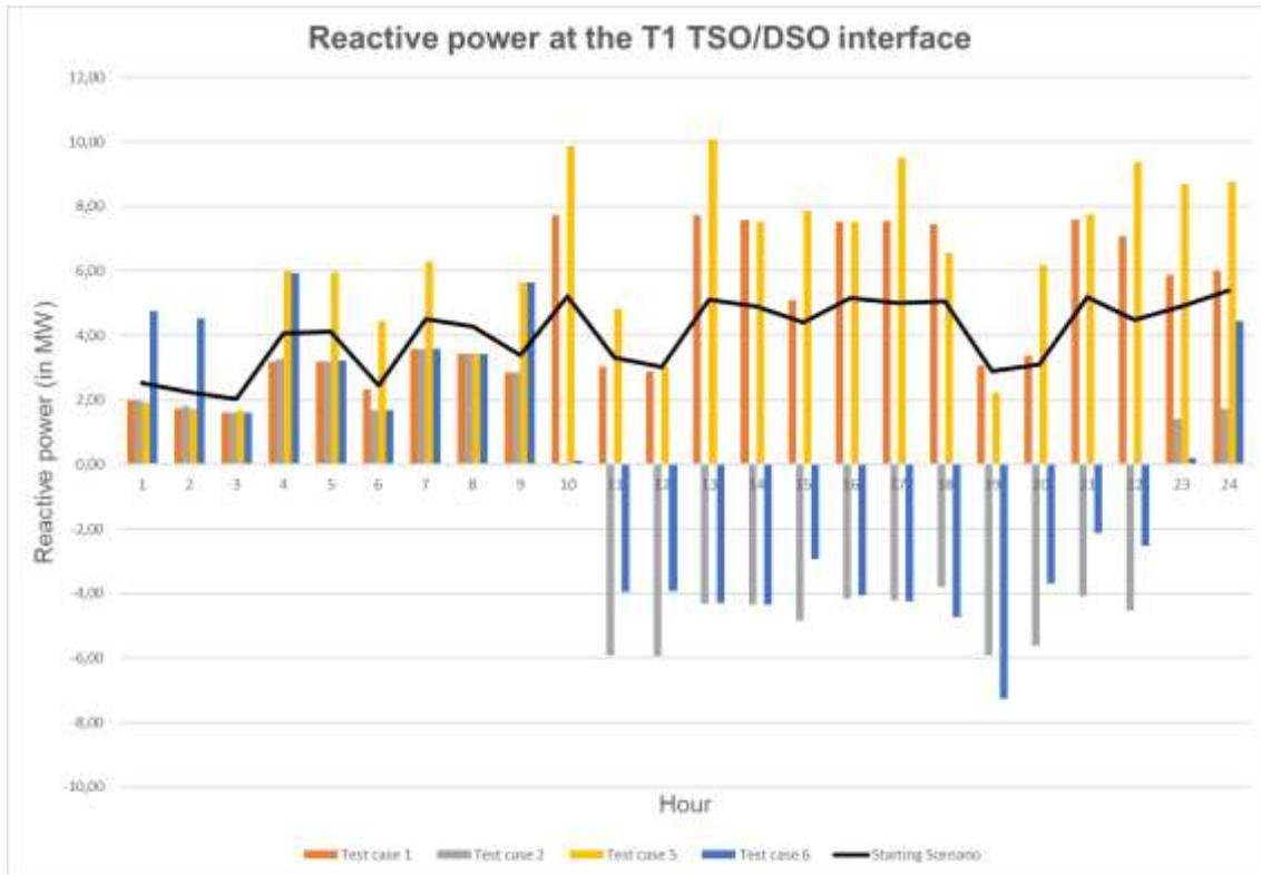
Figure 5-4 – Reactive Power profile at T1 TSO/DSO interface for cluster 1 test cases
