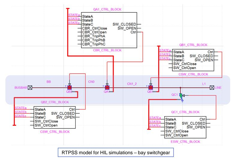
RTPSS model for HIL (Hardware in the loop) simulation – <u>bay switchgear</u>
