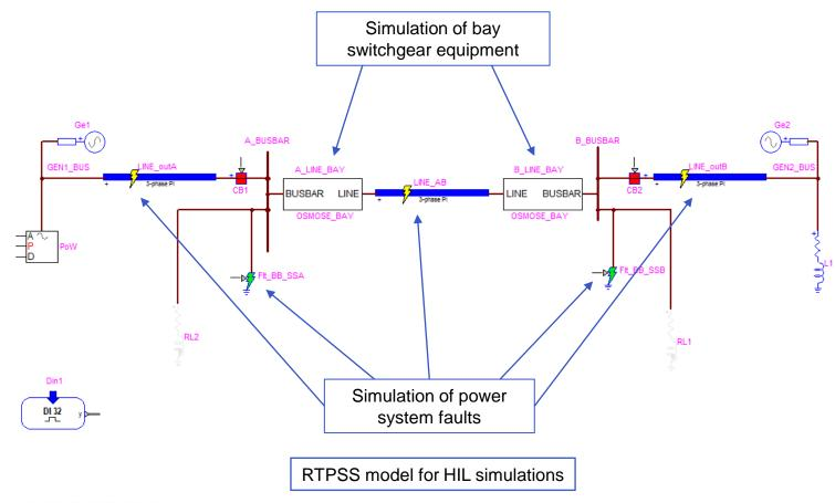
**RTPSS model for HIL (Hardware in the loop)** simulation
