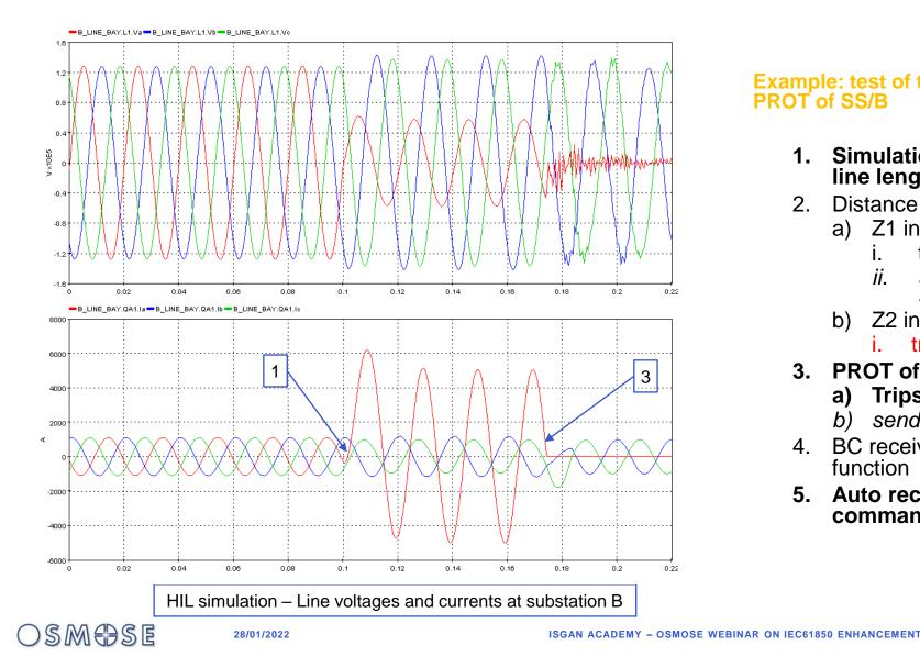
Example: test of trip by <u>teleprotection</u> function by PROT of SS/B
