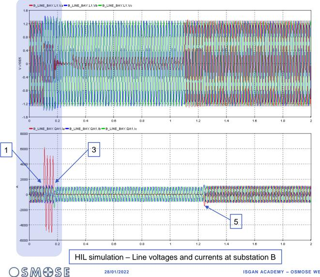
Example: test of trip by <u>teleprotection</u> function by PROT of SS/B
